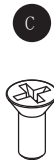
Mounting Screw Qty: 3 pcs +1 Extra 7MPF0412S1 (AL) 7MPF0412S1BK (BK) 4MPF0412S2BB1 (AB) 5/32-32x1/2
