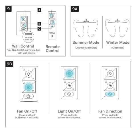
**Fan On/Off**: Press and hold  $\bigotimes$  button for 4 seconds. The LED on the remote will flash green and all connected fans will beep to indicate the message has been received. All fans will turn off. This will bring all fans controlled by the remote into sync.
