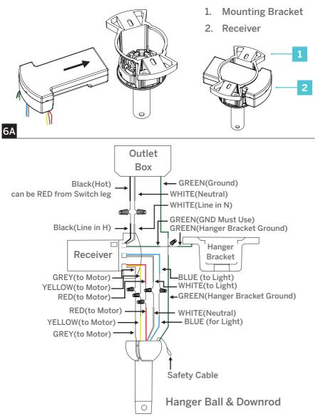
Follow the steps above to connect the fan to your household wiring. Use the plastic wire nuts with your fan. Secure the plastic wire nuts with electrical tape. Make sure there are no loose strands or connections. Failure to do so may result in damage to the electronics.
